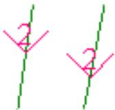
If the symbol points down as shown, the groove is to be cut into the same side as viewed. If the symbol points up, the angle will be greater than 180 and the groove is to be cut on the opposite side.
